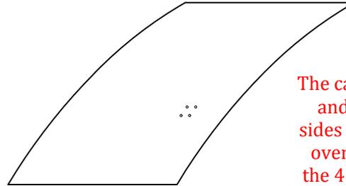
The cab roof 15 is curved to shape and soldered to the top of the sides and front, the front and rear overhangs should be equal and the 4 rivets in a square should be to the right nearer the front.
