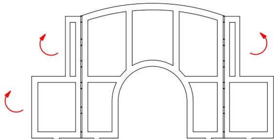
Cab front frame 2, fold sides back 90 degrees and solder into slots in the floor
