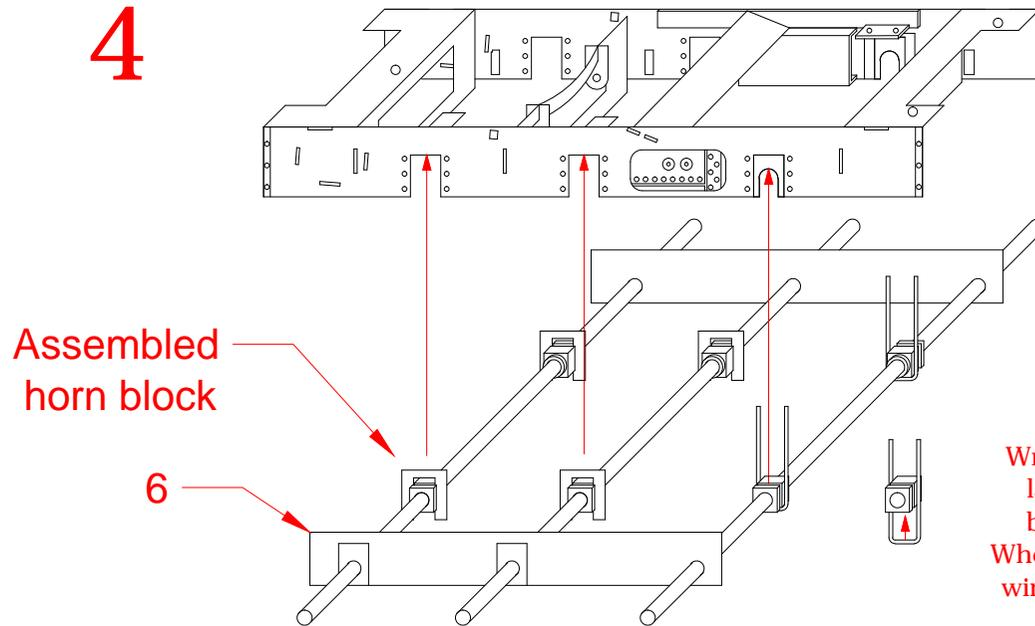
Assemble like this, shown here with long axles for clarity. If you can find springs to fit between the horn blocks they will hold things in place during soldering. Do all this with the frames upside down.
