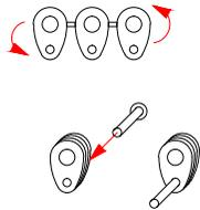
Cut out the cranks in threes, fold into a zig-zag and solder. Countersink the small hole and solder a 1mm screw into it. File the back flush and open out the large hole until it just fits on the axle. Clean up all round with files.
