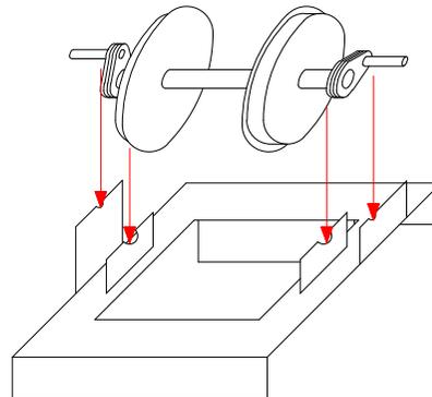
Assemble the quartering jig to the gauge you are using, 12mm builders will have to file the tags off the axle supports in position them 1mm nearer the middle. Assemble all the parts onto the axles, the rear axle has the gearbox already fitted. Solder one crank to one end of each axle. Position one axle in the jig with the crank vertical, put the other crank in place and oil the axle supports. Flux the outside of the crank and solder in place.
