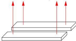
PCB for pick ups, glued to folded over strips on front and centre spacers
