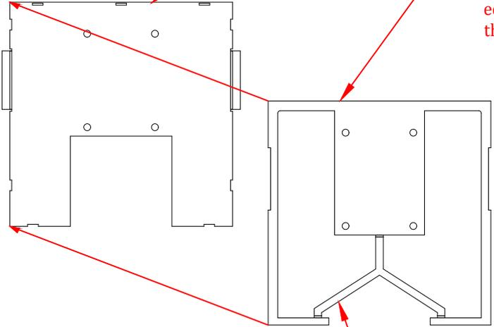
Remove this Y piece after the edges are soldered
