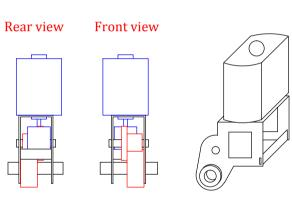
This is what the 14/16.5mm gearbox should look like, the 12mm one has the same layout but the gears are between the frames. Motor and worm are shown in blue and the reduction gears in red.
